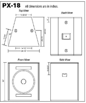
forced with 16-gauge steel plates and connected together with 1/4" threaded rod to facilitate rigging one enclosure to another.
